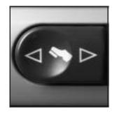
The switch used to adjust the pedals is located on the left side of the instrument panel.
